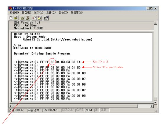
0xFE is BROADCAST\_ID, so Dynamixel does not return status packet.(First 2 Instruction Packet)
